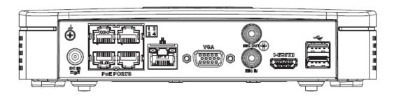
The NVR41-8P-4KS2/NVR41-8P-4KS2/L/NVR41-8P-4KS2/H/NVR21-8P-S3 series rear panel is shown as below.
