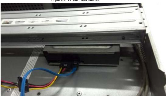
Figure 3-41 Connect cables
