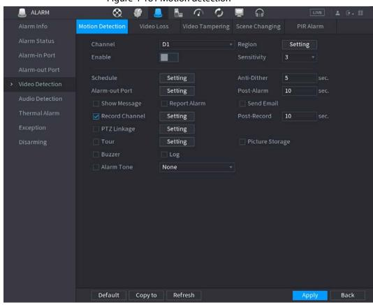
Figure 4-181 Motion detection
