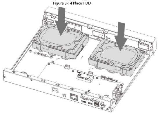
Step 4 Turn the device upside down, match the screws with the holes on the HDD and then fasten them. The HDD is fixed to the baseboard.
