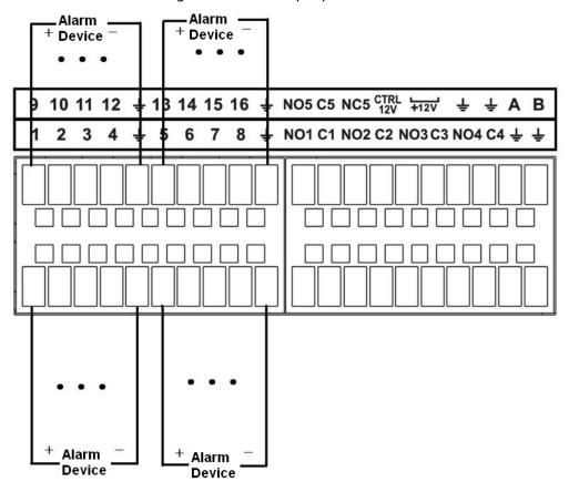
Figure 2-81 Alarm input port
