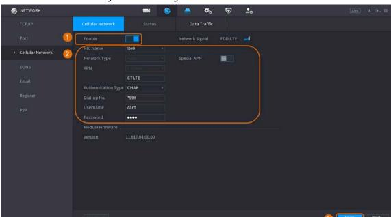
Figure 4-220 Configure cellular network
